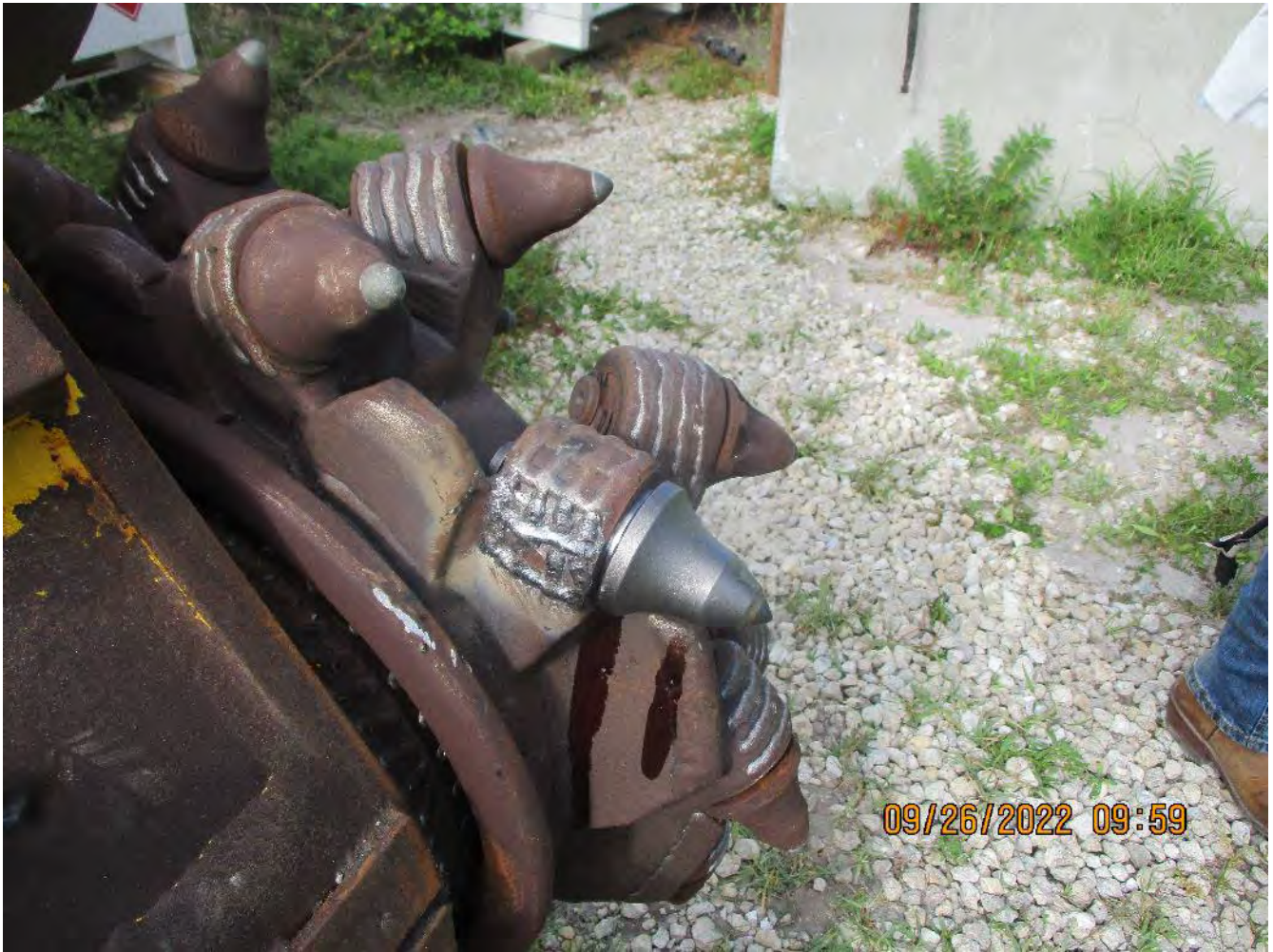
Repaired sleeve area and new tooth in place
