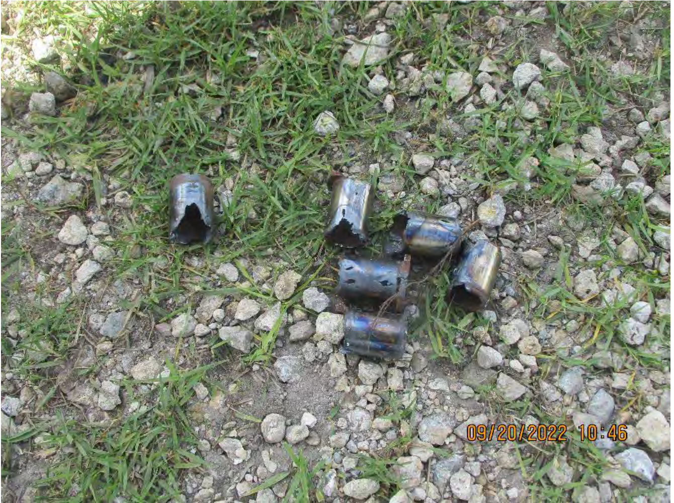
Removed worn bushings from grinding attachment teeth locations
