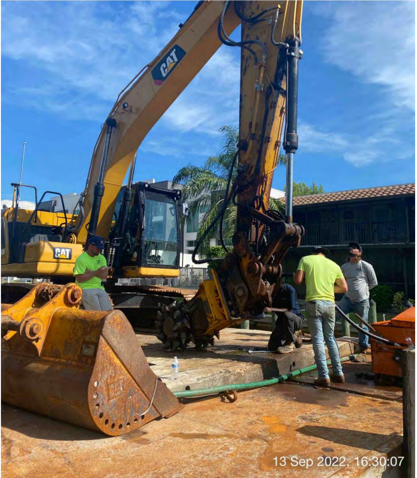
Mechanic replacing hydraulic hose on 323 excavator
