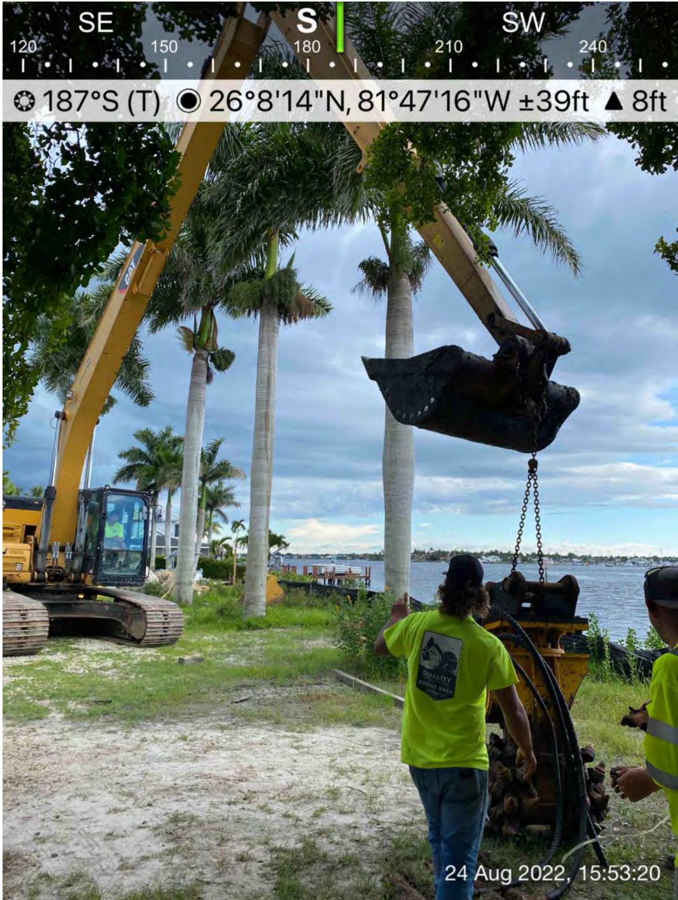
326 excavator lifting Epiroc grinder
