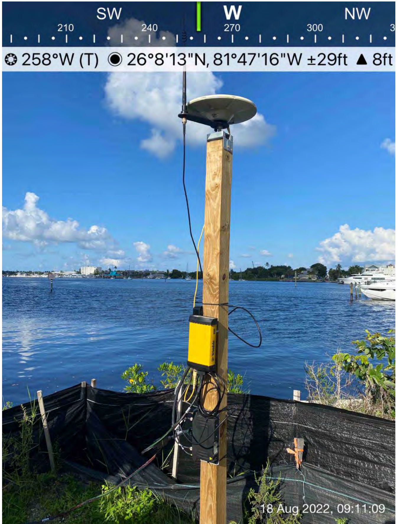
Trimble base station at southwest corner of 1300 Curlew Avenue
