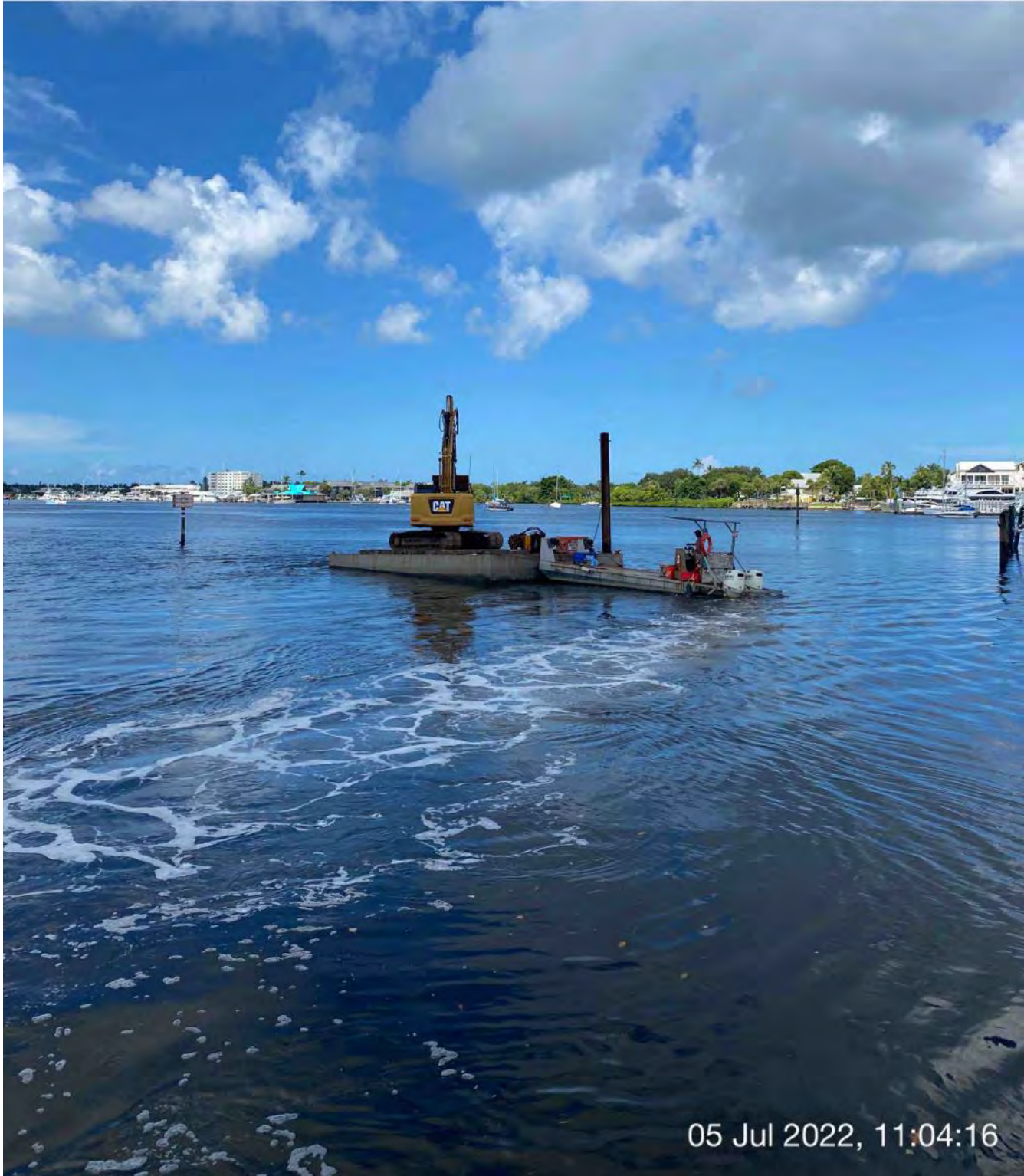
Contractor using push boat to transport barge and 323 excavator from Canal CC-CC to Canal X-X
