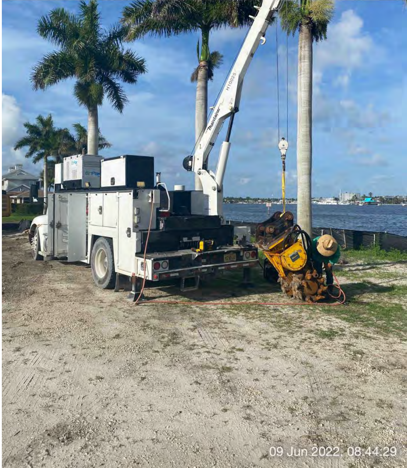
Contractor using Utility truck to lift Epiroc grinder in order to fix the bearing on one of the teeth
