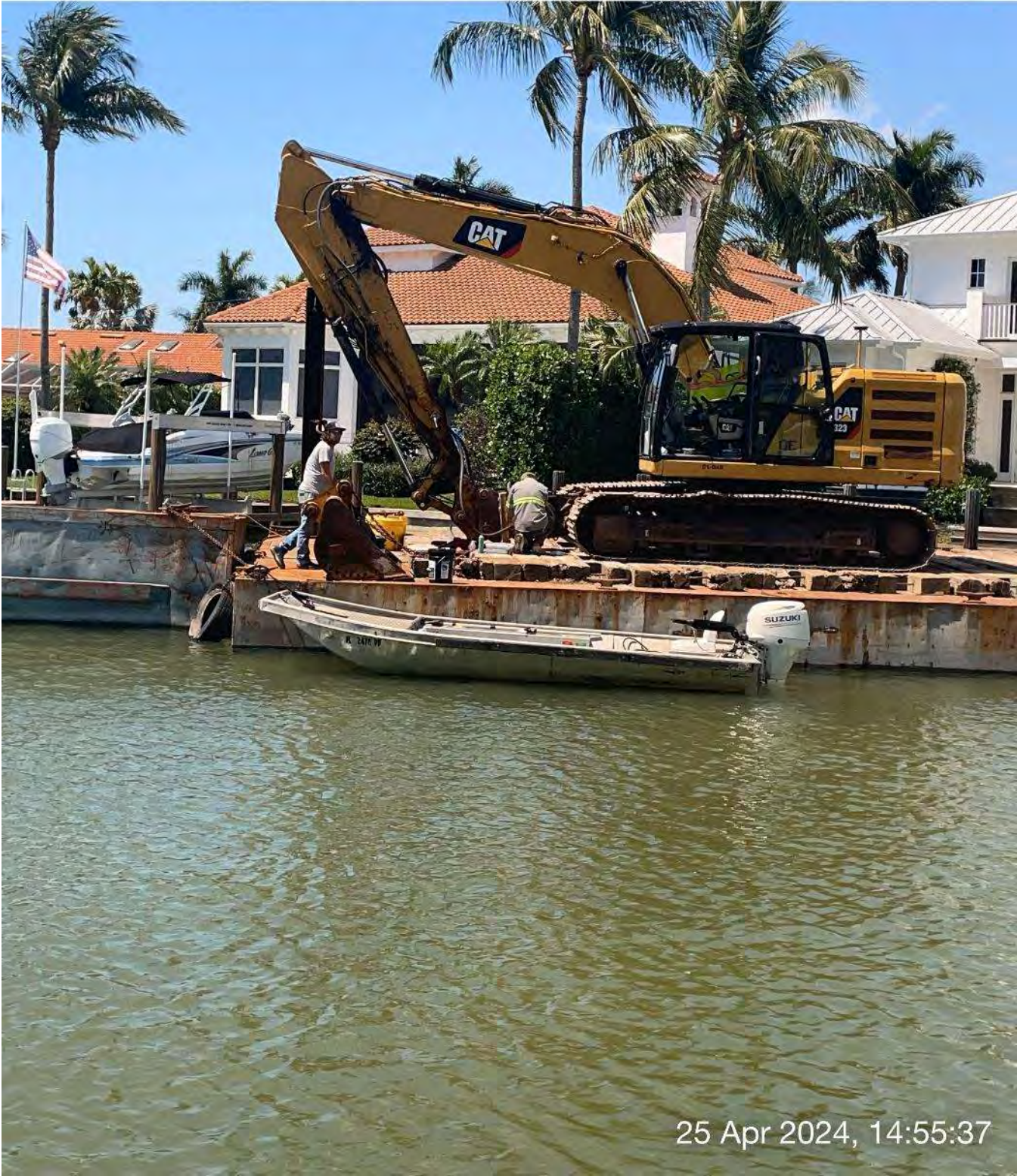
Mechanic repairing hydraulic lines on 323 excavator.
