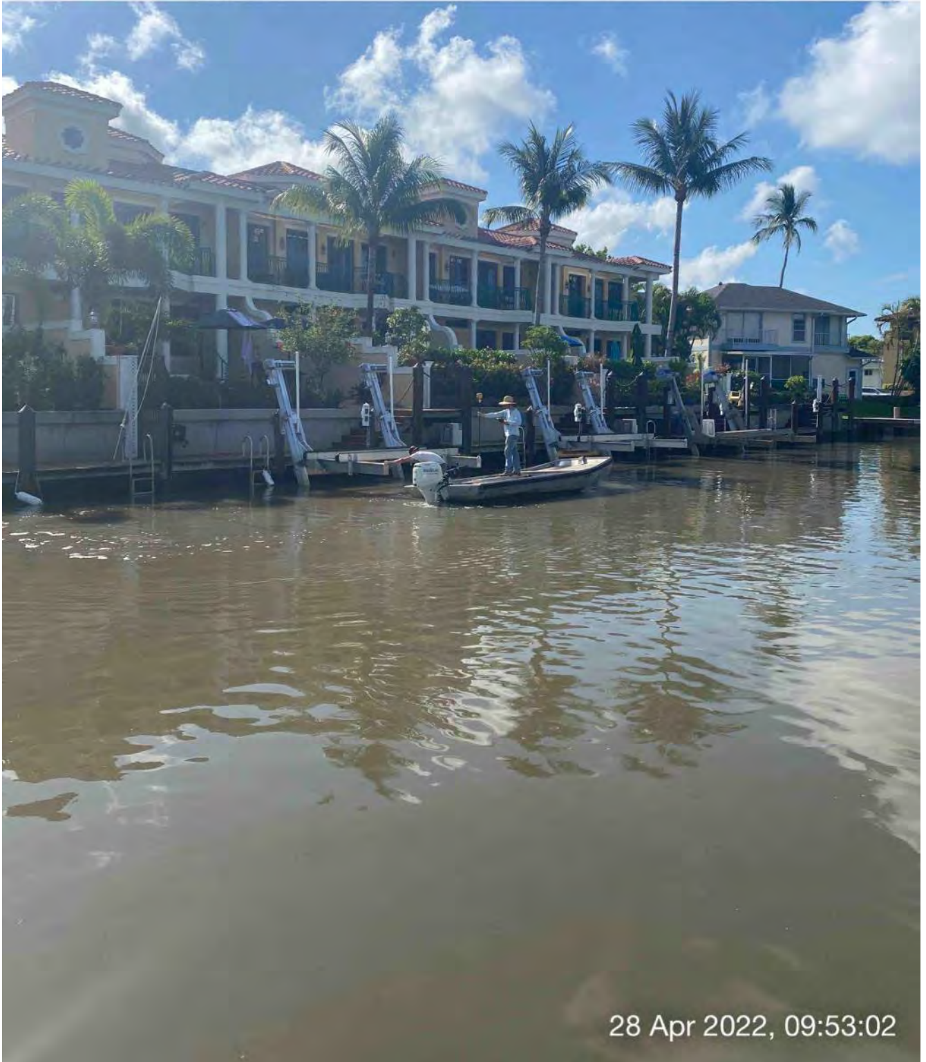
Using support boat and RTK Trimble GPS unit to map locations of existing boat lifts at station 3+00
