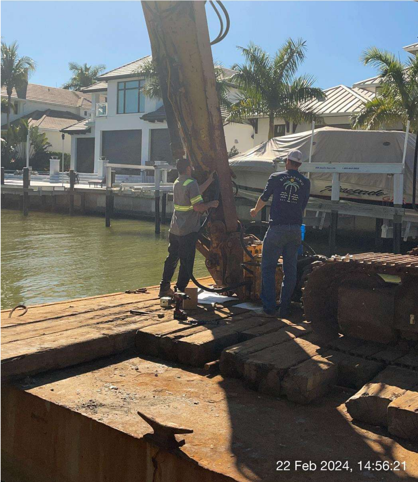
Mechanic working to disconnect Epiroc grinder from 323 excavator.
