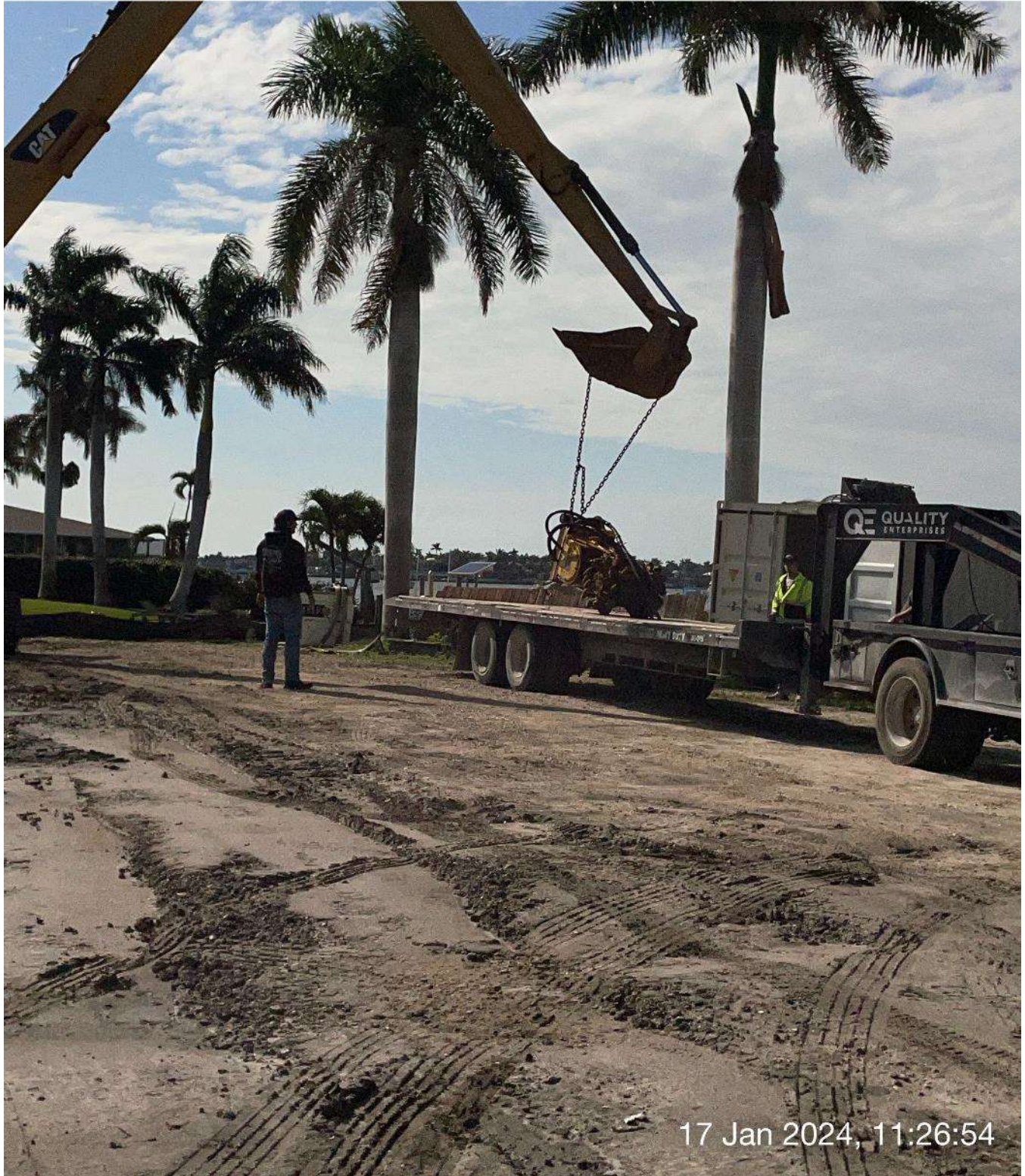
Long reach excavator loading Epiroc grinder onto trailer.
