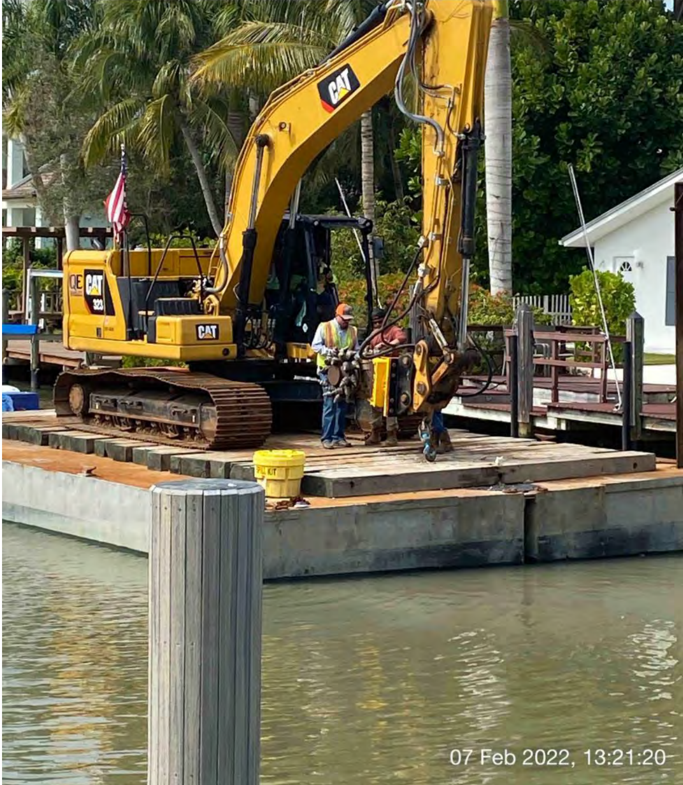
Inspecting and replacing teeth on the Epiroc grinder
