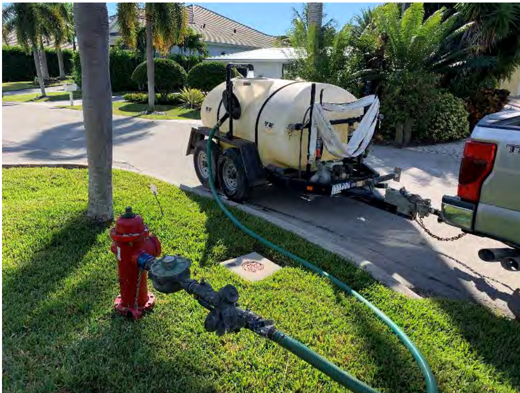
Water trailer being filled at West end of Curlew.
