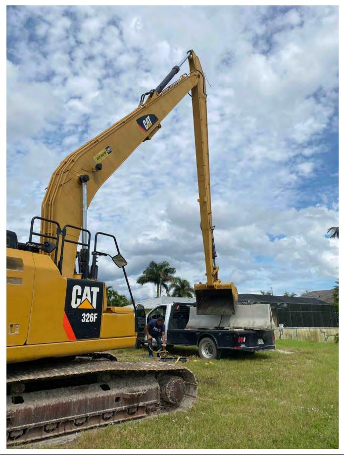
• 326 excavator positioning barrier element in empty lot staging area.
