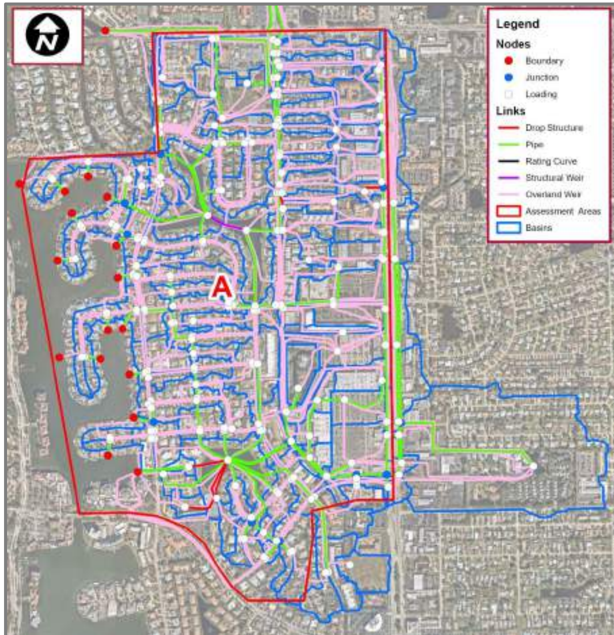
Figure 3-5 North Model Existing Conditions Schematic
