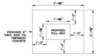
THIS ASSEMBLY IS RATED FOR A STATIC DESIGN LOAD OF 15,000 LBS. OVER A 10 X 10 AREA AND MUST PASS A MINIMUM STATIC TEST LOAD
