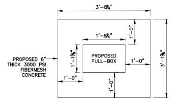
THIS ASSEMBLY IS RATED FOR A STATIC DESIGN LOAD OF 15,000 LBS. OVER A 10 X 10 AREA AND MUST PASS A MINIMUM STATIC TEST LOAD
