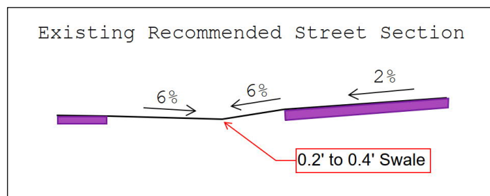
Figure 19. Existing Standard Swale
