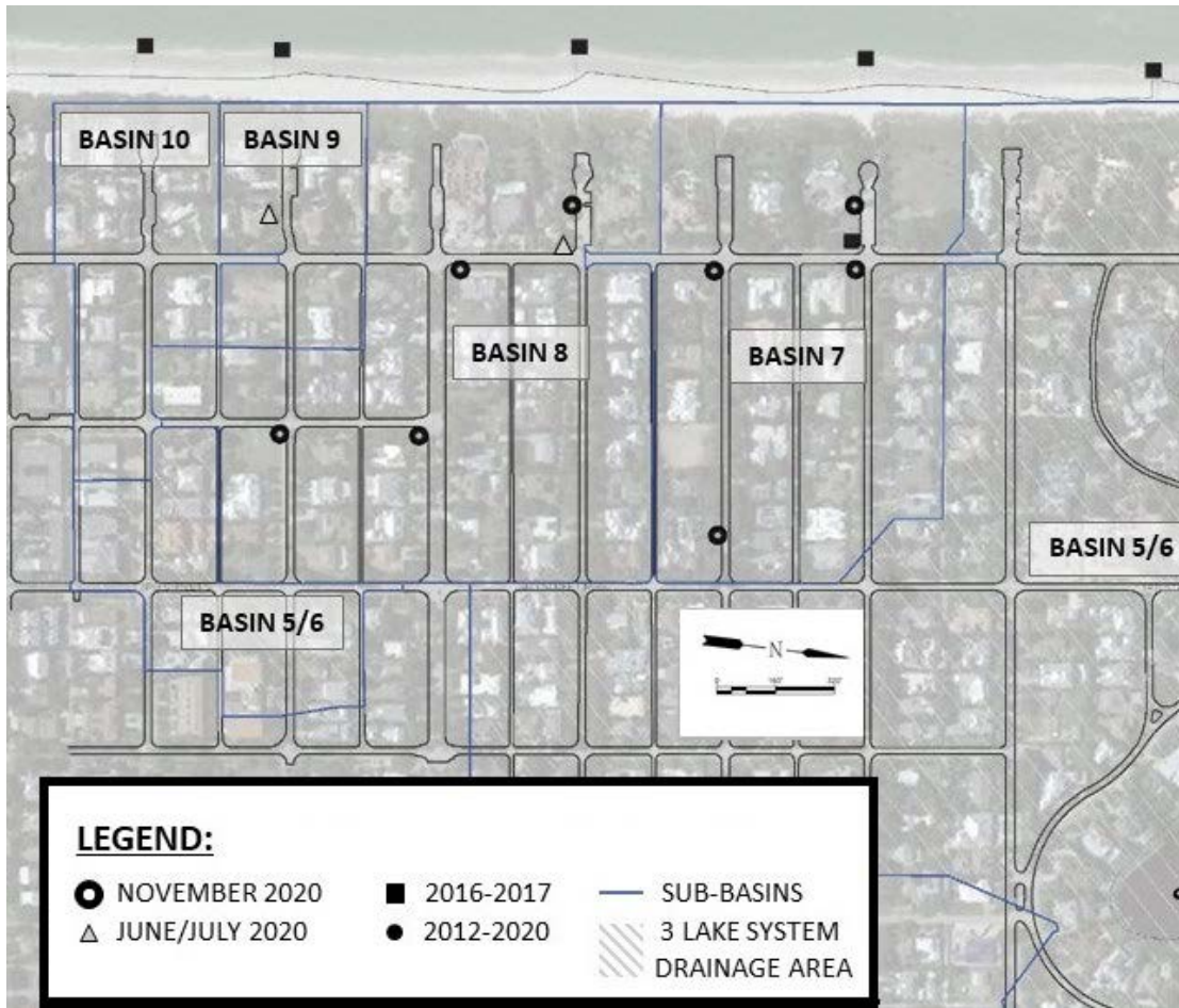
Figure 1. Water Quality Sampling Locations. 2020 Sampling locations to be repeated, and additional inlets in Basins 7, 8 and 9 will be identified on site based on rainfall conditions. At least one inlet in Basin 7 should be upstream of 3 rd Street to capture the water quality further from the beach outfalls.
