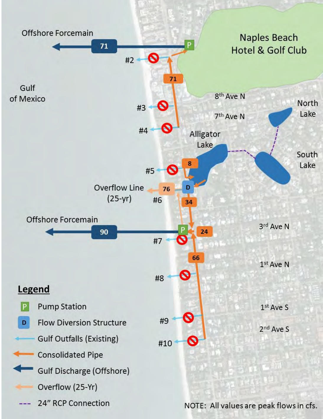
Figure 4-3. Alternative 3: Conceptual Flow Schematic
