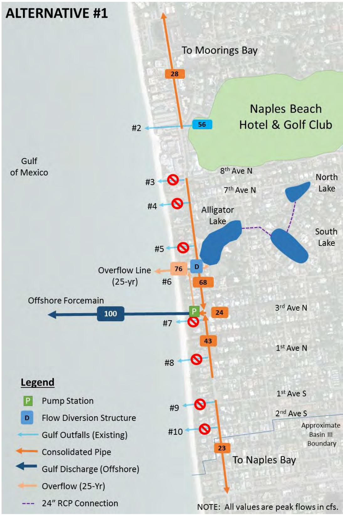
Figure 4-1. Alternative 1: Conceptual Flow Schematic
