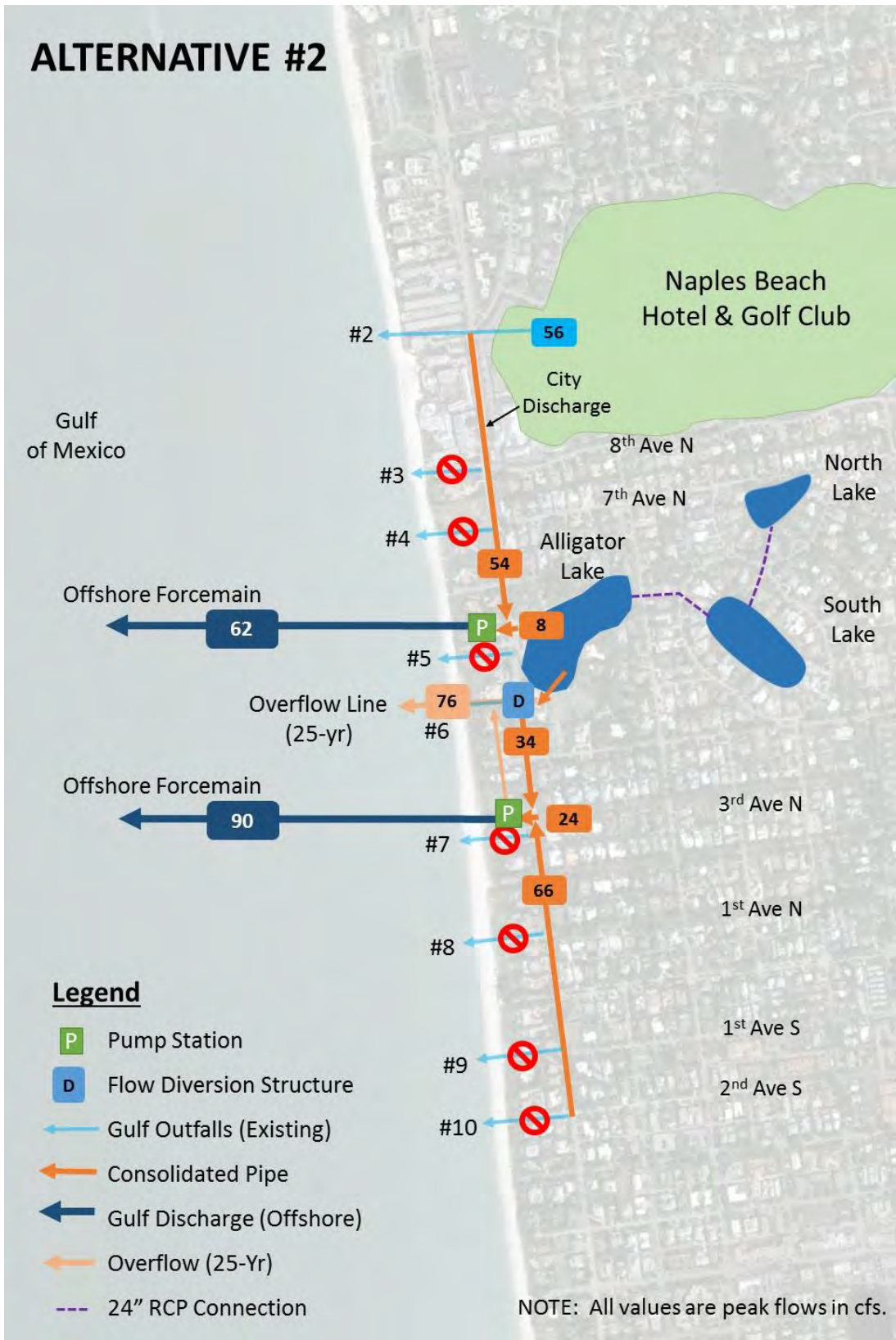
Figure 4-2. Alternative 2: Conceptual Flow Schematic
