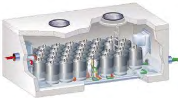
Figure 3-20. Typical Media Filter
