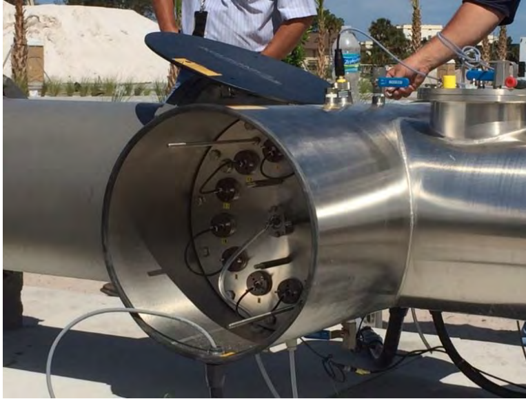
Figure 3-21. Typical Inline UV Reactor Unit
