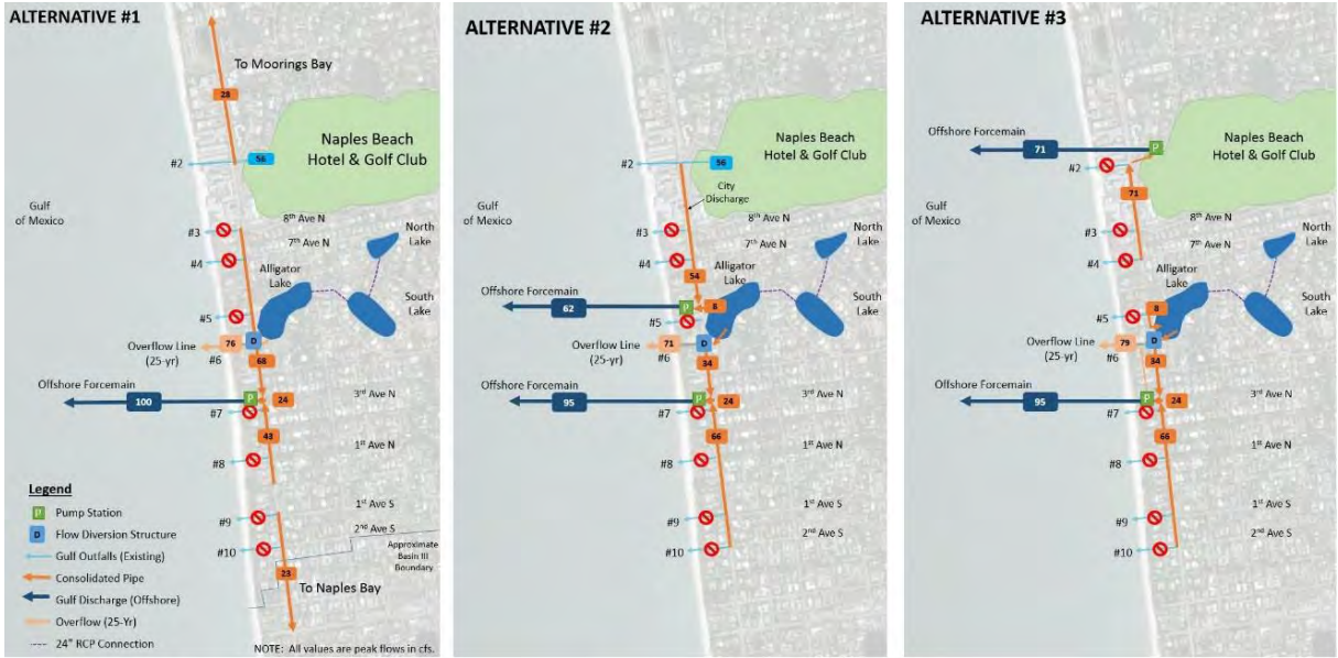
Alternative 1: Single Pump Station @ 3 rd Ave N
