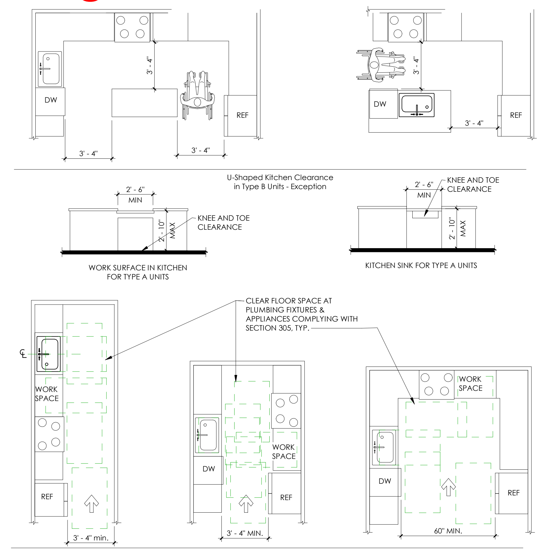
FIGURE 1103.12.1.1, 1104.12.1 MINIMUM KITCHEN CLEARANCE IN A & B TYPE UNITS
