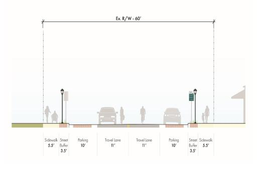
Includes sidewalks on both sides, striping on the roadway which represents that the travel lane is to be shared between bicyclists and vehicles, and parallel parking on both sides.
