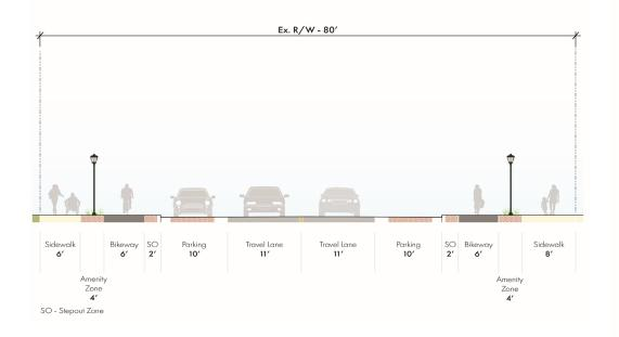
Includes a raised bikeway which is separated from the roadway. Also included is a sidewalk adjacent to the raised bikeway separated by an amenity zone and parallel parking on both sides of the street.
