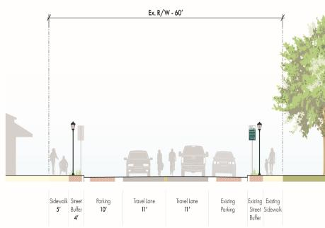
Includes sidewalks, striping on the roadway which represents that the travel lane is to be shared between bicyclists and vehicles, and parallel parking on both sides.
