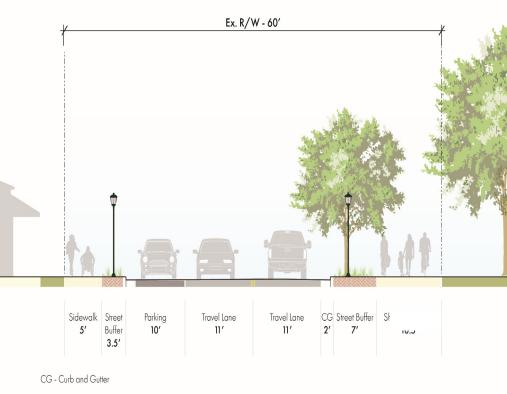
Includes sidewalk on west side, shared use path on east side and parallel parking on west side.
