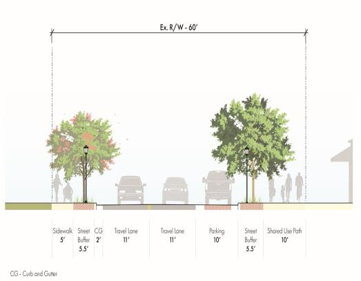
Includes sidewalk on west side, shared use path on east side, and parallel parking on east side.
