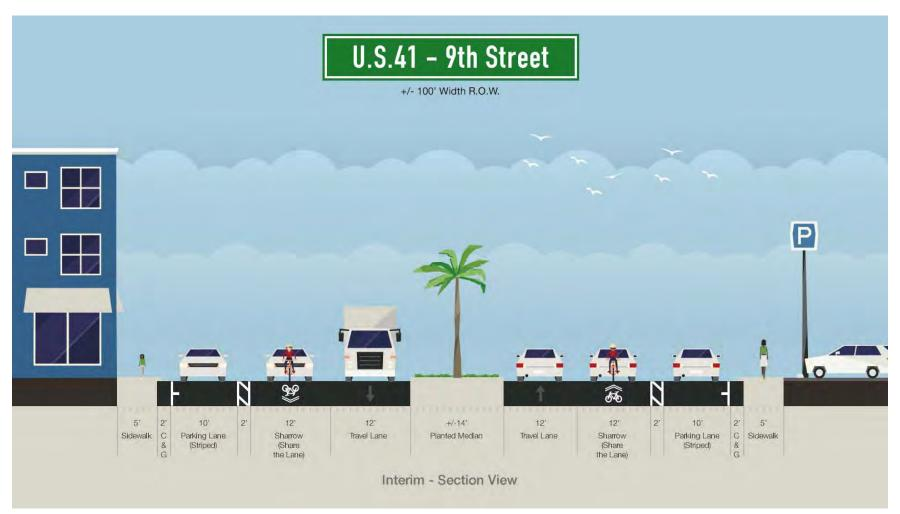
Figure 3-2 US 41/9<sup>th</sup> Street- Interim Improvements Plan Section View
