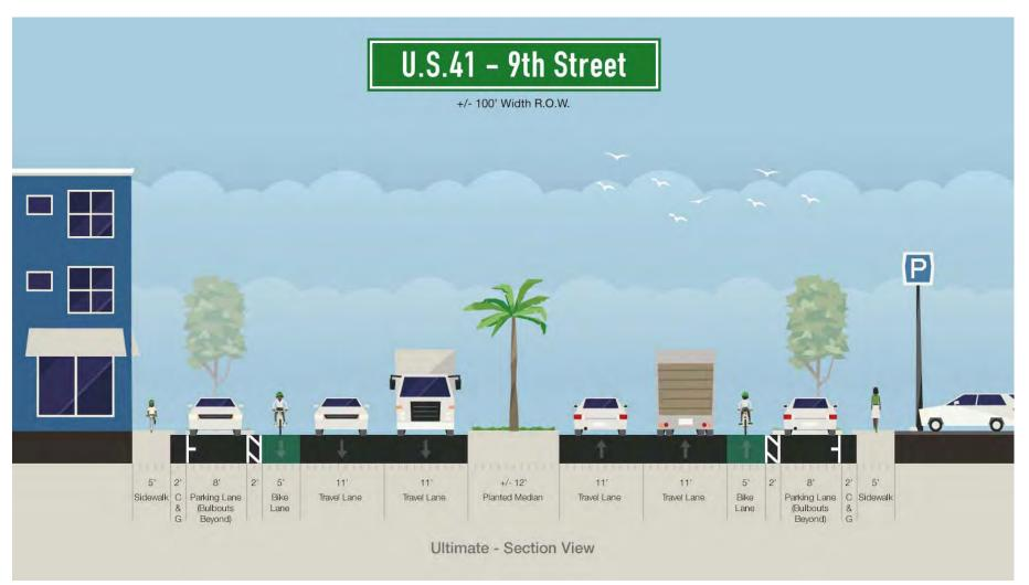
Figure 3-5 US 41/9<sup>th</sup> Street- Ultimate Improvements Section View
