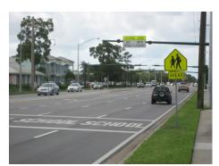
The two (2) primary roadways for ingress and egress are US 41 and Goodlette-Frank Road. US 41/Tamiami Trail is a 6-lane divided principal arterial with a north-south direction and a posted speed limit varying from 30 MPH to 40 MPH within the study limits. Available data indicate US 41 accommodates an average daily traffic ranging between 29,000 and 36,500 vehicles per day. Within the limits of the
