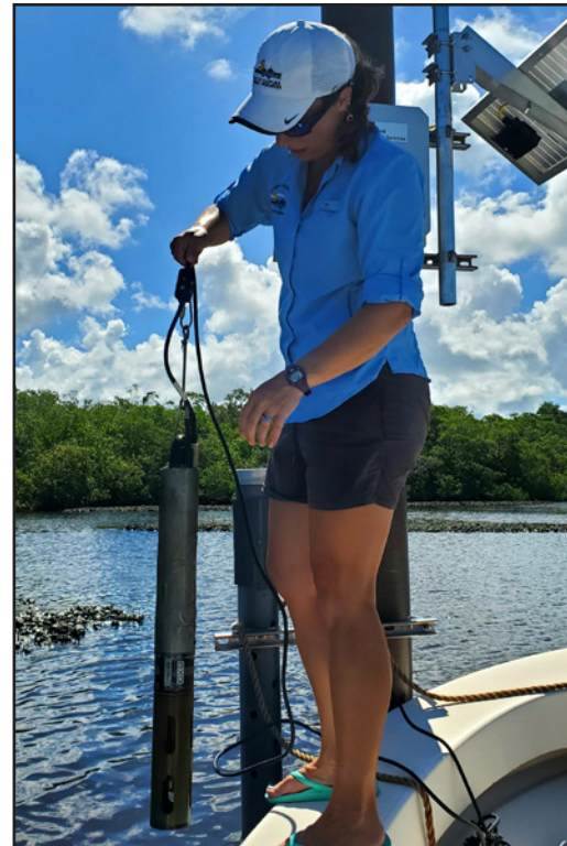
Checking the continuous datasonde which measures water quality every 15 minutes at Site 1.
